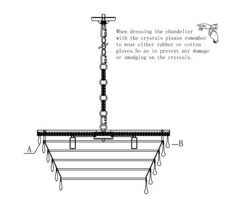
1. Hang the crystal (A) and the crystal (B) on the first circle to the sixth circle of the Lamp Frame as shown in the figure.
